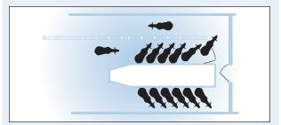
A carousel, or rotary, milking parlour moves the cows around so that the farmer can stay in one place to attach the milking machine.
