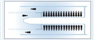
In a herringbone milking parlour, cows are lined up at an angle. This makes it easier for the milking machine to be attached and the cows to be milked.
